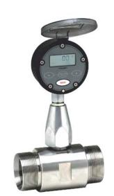
Standard version of the device has a frequency output (mV sinusoidal waves) or a preamplifier output of the square waves (4...20 mA impulses). Turbine type flowmeter has a MS terminal for the impulse signal output. It can also be equipped with the integral devices for the operating in adverse conditions that can amplify the signals' transmission range or connect to the accessory instruments that require a corresponding input signal.
